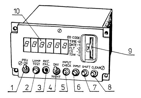
Fig. 7 - 48 Control panel PU 25
