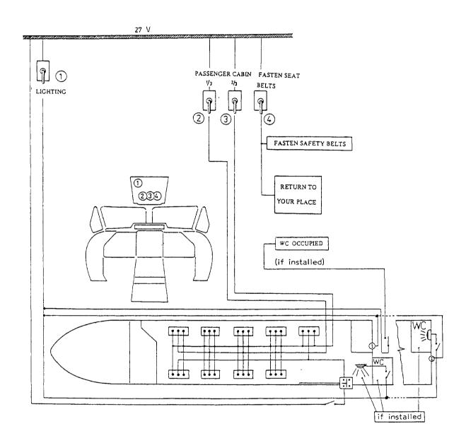
Fig. 7 - 34 Passenger compartment lighting
