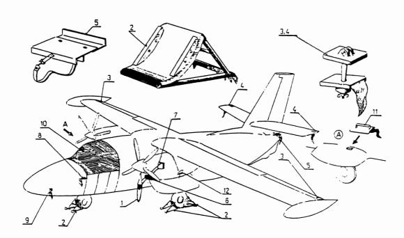
Fig. 8 – 4 Parking equipment for parking on the apron
