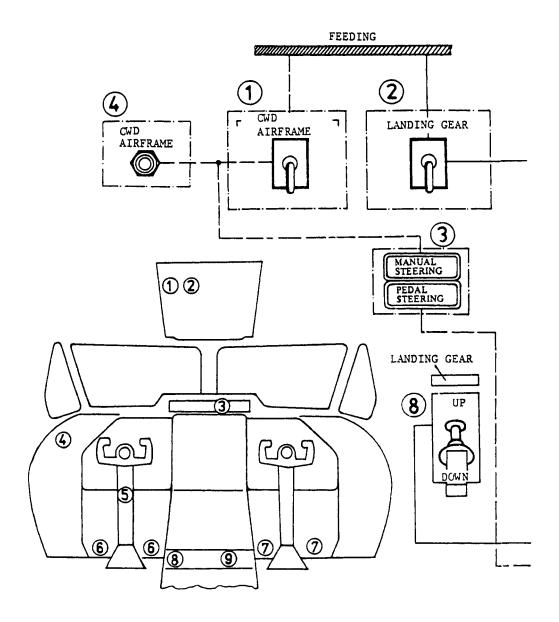
Fig. 7 - 20 Nose landing gear steering
