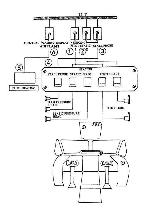
Fig. 7 - 39 Heads pressure deicing
