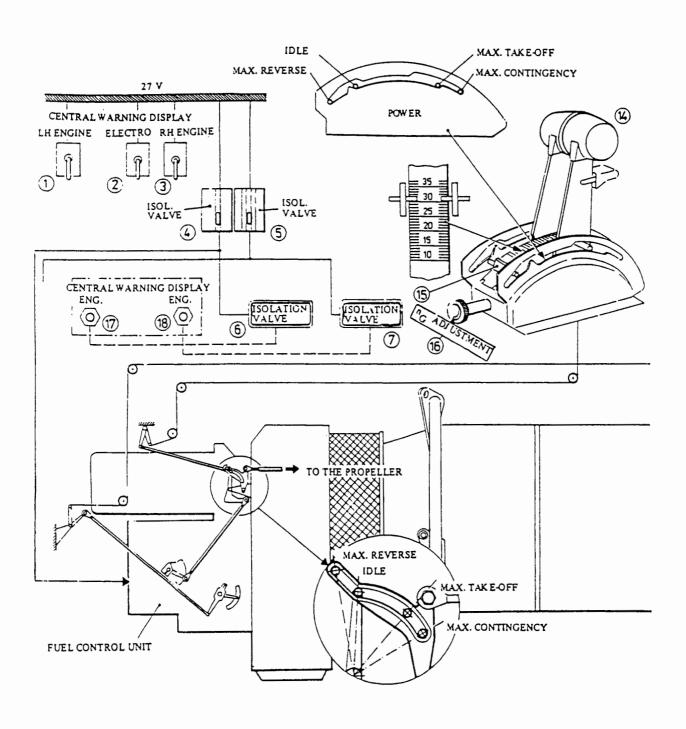
Fig. 7 - 25 Power unit controls
