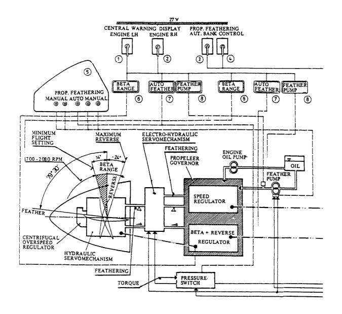
Fig. 7 - 27 Propeller control system
