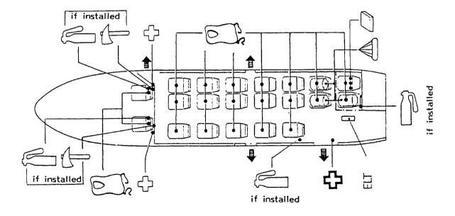
Fig. 7 - 50 Emergency equipment location
