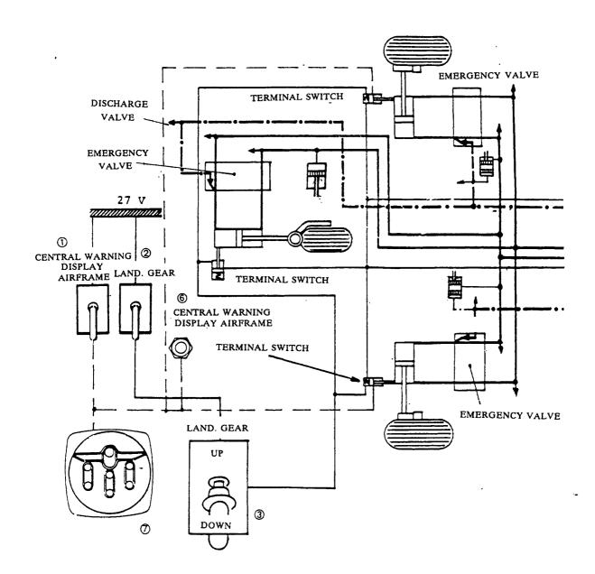
Fig. 7 - 19 Landing gear extension and retraction
