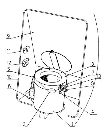
Fig. 8 - 9 Toilet with collecting vessel
