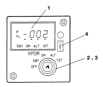
Fig. 1 - Control box of KXP 756
