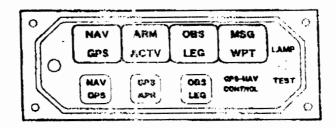
Fig. 2 MD~41 GPS Annunciation control unit
