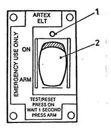
Fig. 2 ELT's Remote Switch Panel
