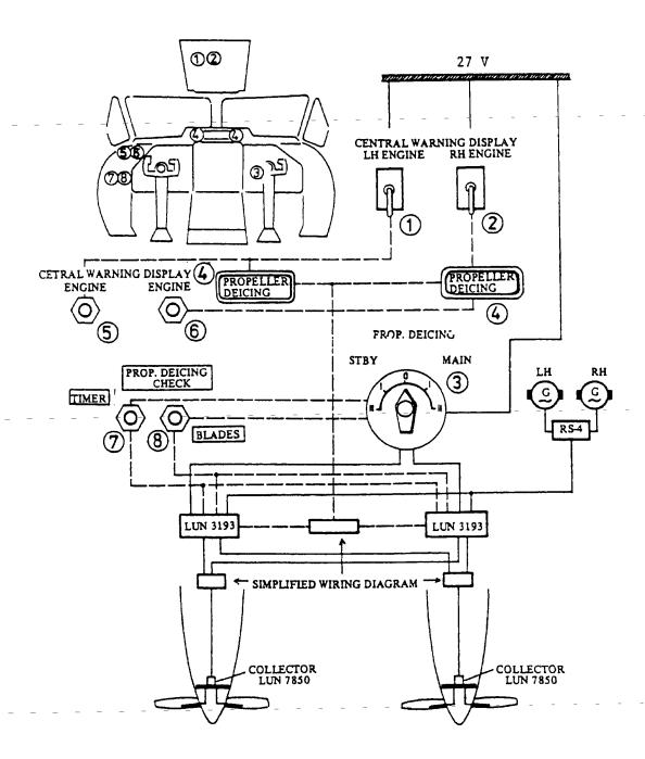
Fig. 7 - 41 Propellers deicing
