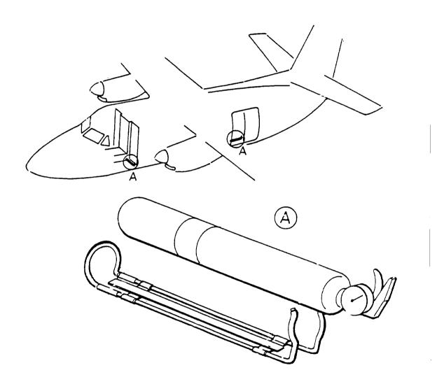
Fig. 7 – 42 Location of portable fire extinguishers
