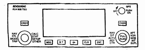
Fig. 1 KLN 90B Control panel
