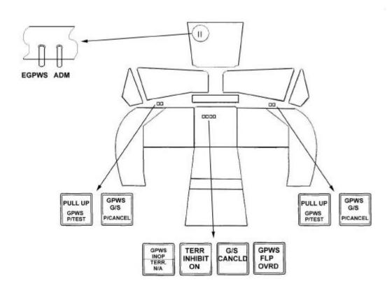
Fig. 1: EGPWS switches and annunciators
