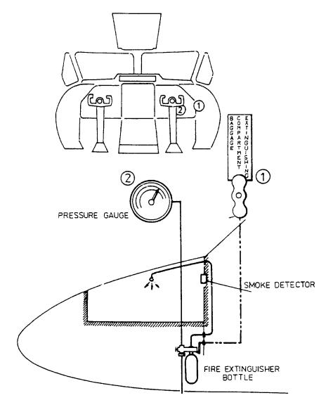
Fig. 7 – 46 Baggage compartment fire extiguishing system
