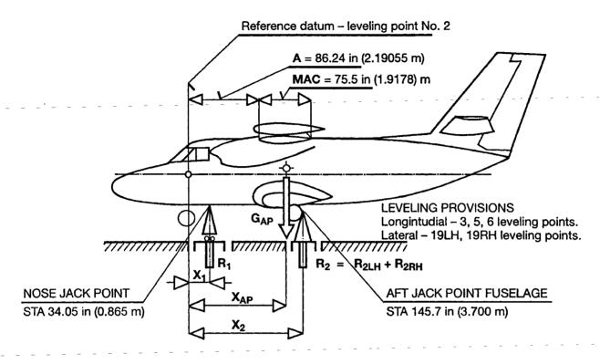
STA - Station, a position along the fuselage measured from reference datum.
