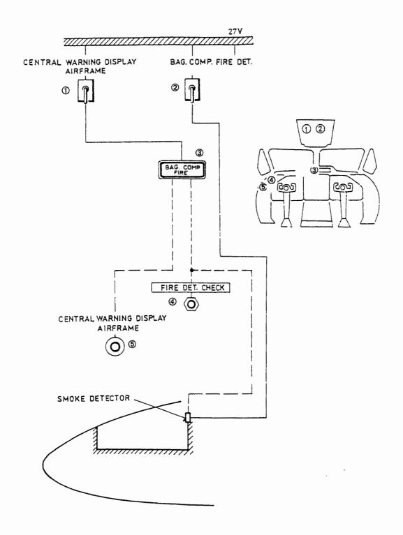
Fig. 7 - 45 Baggage compartment fire detection
