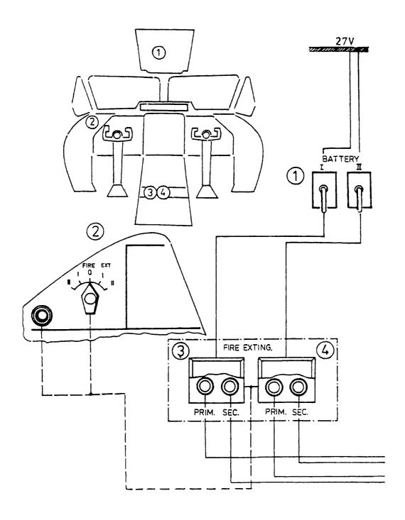
Fig. 7 – 44 Engine fire exextinguishing system
