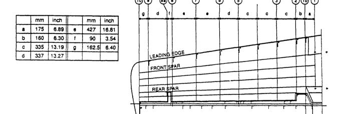
Fig. 7 – 4 Horizontal Stabilizer and Elevator Station Diagram
