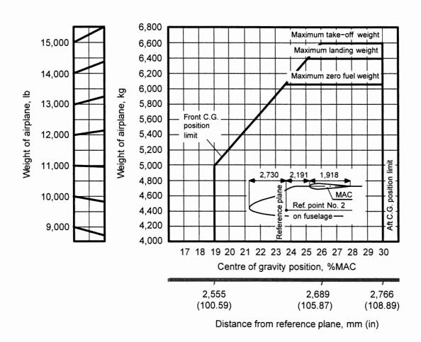
Fig. 2 - 1 CENTREOF GRAVITYLIMITS AND MAC POSITIONS
