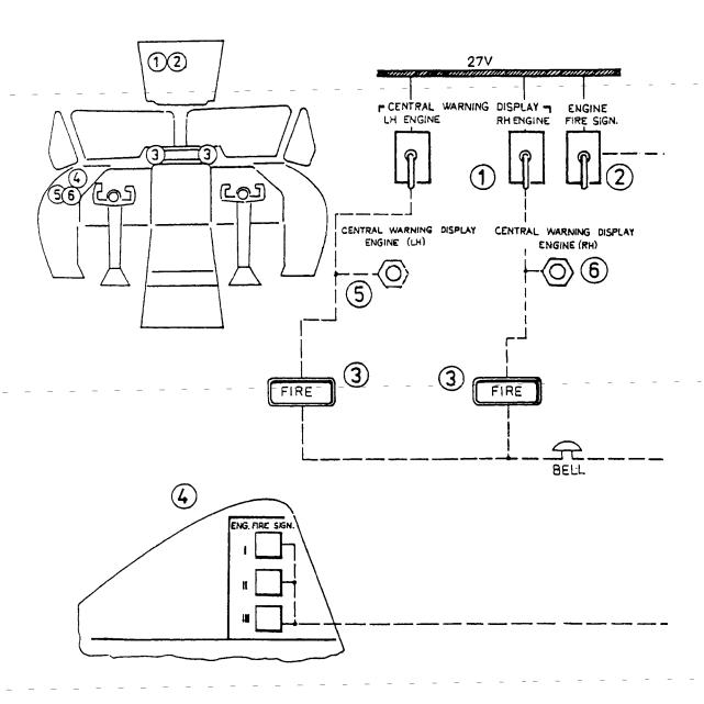
Fig. 7 - 43 Engine nacelle fire detection system
