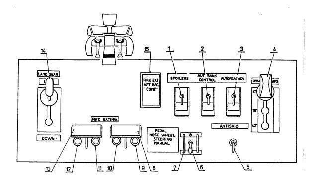
Fig. 4 Central control panel
