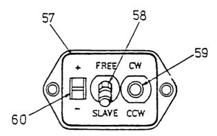
Fig. 5 KA 51B SLAVING ACCESSORY AND COMPENSATOR UNIT
