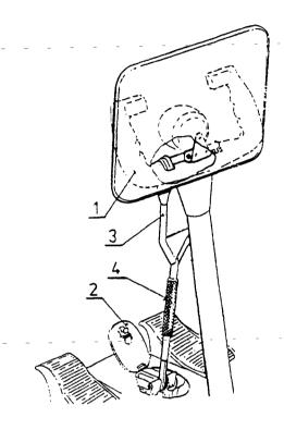
Fig. 8 - 3 Securing of column by blocking strut
