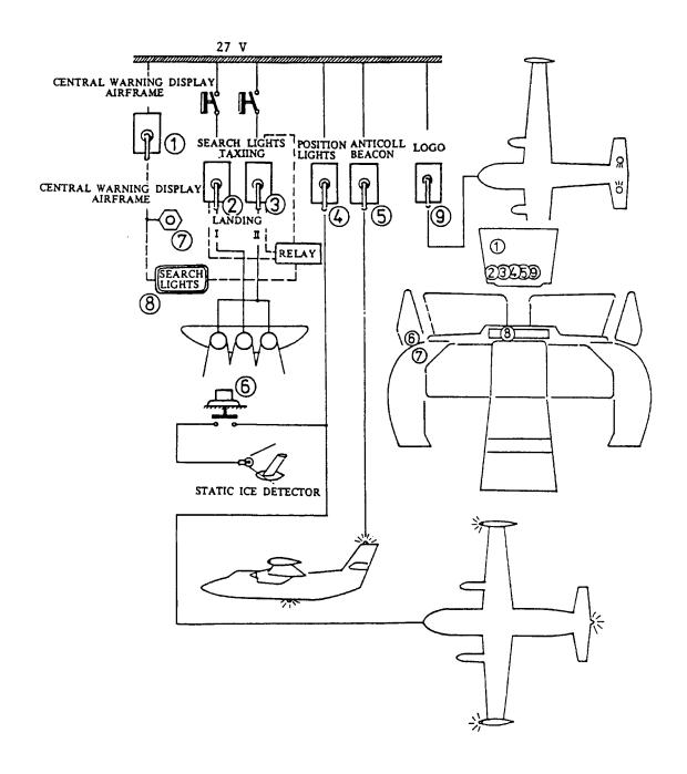
Fig. 7 - 32 Light system exterior
