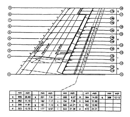
Fig. 7 - 3 Vertical Stabilizer and Rudder Station Diagram
