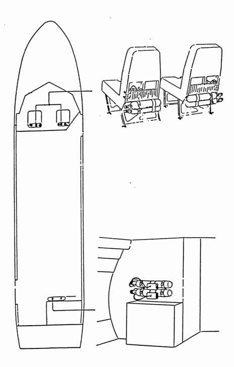
Fig.4 - Location of the oxygen equipment
