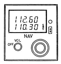
Fig. 1 - Control box of KNR 634
